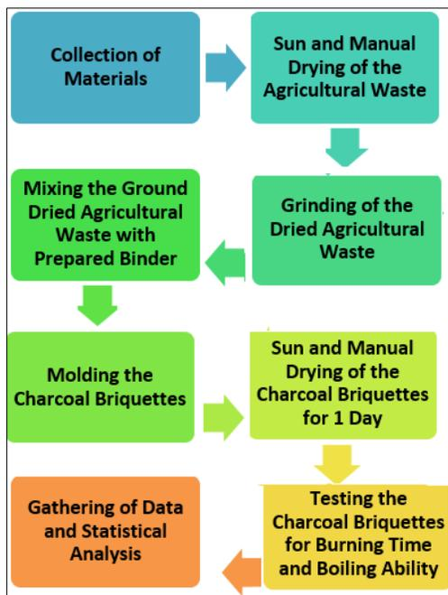
Fig 1: Process flowchart
